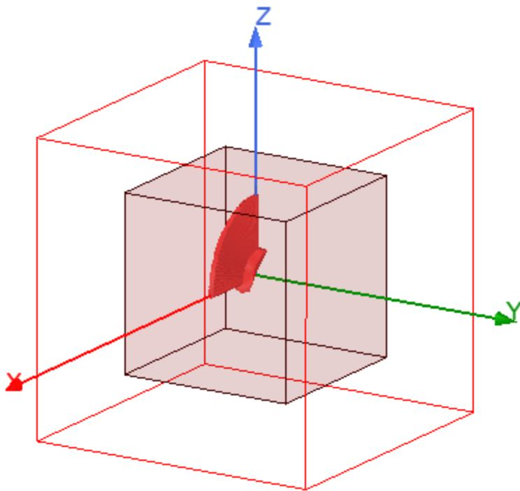
The radar cross-section (RCS) or echo area,  $\sigma$ , is measured in meters squared and represented for a bistatic arrangement (that is, when the transmitter and receiver are in different locations as shown in the figure below).
