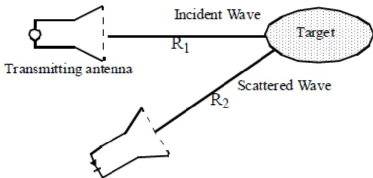
HFSS supports RCS for Bistatic, Normalized Bistatic, Complex Bistatic, and Monostatic conditions. In this tutorial, you will generate plots for Normalized Bistatic and Monostatic situations.
