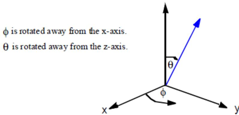
When HFSS evaluates the radiated fields, it needs at least two directions along which to plot the fields. Therefore, if the step size for phi is zero, then the step size for theta must be greater than zero, and vice versa, which ensures that the fields are plotted in at least two directions.
